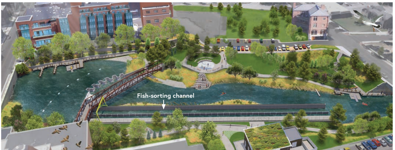
A RENDERING OF THE FISHPASS PROJECT, WITH THE FISH-SORTING CHANNEL MARKED ABOVE. IMAGE CREDIT: AECOM
