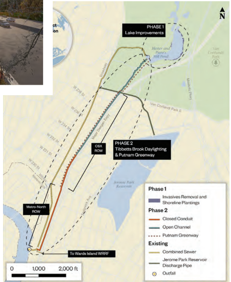
(ABOVE) A MAP HIGHLIGHTS THE SCOPE OF WORK FOR THE TIBBETTS BROOK DAYLIGHTING PROJECT. IMAGE CREDIT: NEW YORK CITY DEPARTMENT OF ENVIRONMENTAL PROTECTION
